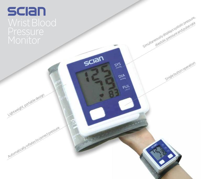
This convenient, portable blood pressure monitor wraps around the wrist and uses the oscillometric principle to simply and accurately measure systolic pressure, diastolic blood pressure and pulse rate.
