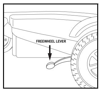
Figure 10. Freewheel Mode (Drive Disengaged)
