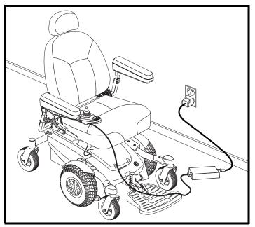
Figure 23. Battery Charging (Select 6 Shown)
