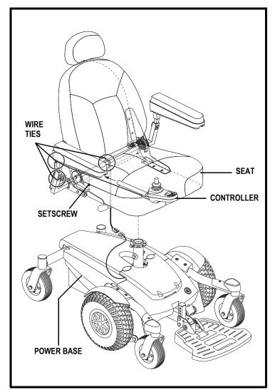
Figure 11. Seat and Controller Assembly
