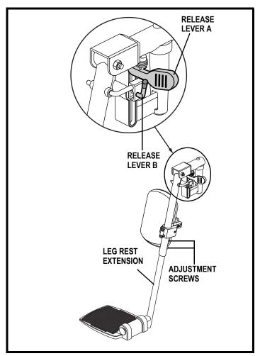
Figure 18. Elevating Leg Rests
