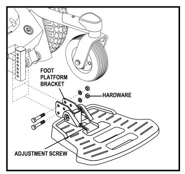
Figure 16. Select 6 Foot Platform Adjustment
