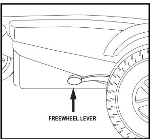
Figure 9. Drive Mode (Drive Engaged)
