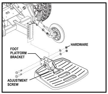
Figure 15. Select Foot Platform Adjustment
