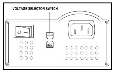
Figure 21. Manual Voltage Switch Off-board Charger
