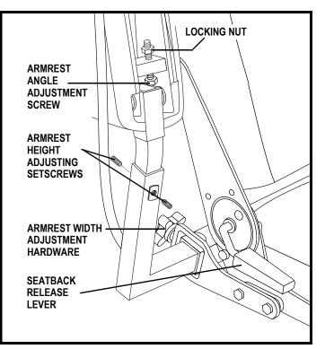
Figure 13. Armrest and Seatback Adjustments
