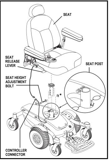
Figure 12. Seat Height Adjustment
