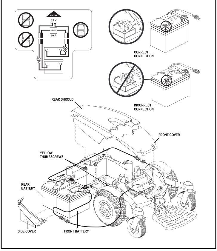
Figure 26. Battery Installation (Seat Removed for Clarity—Select 6 Shown)
